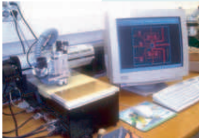
• Manufacturing of prototypes on soft substrates up to 18 Ghz
